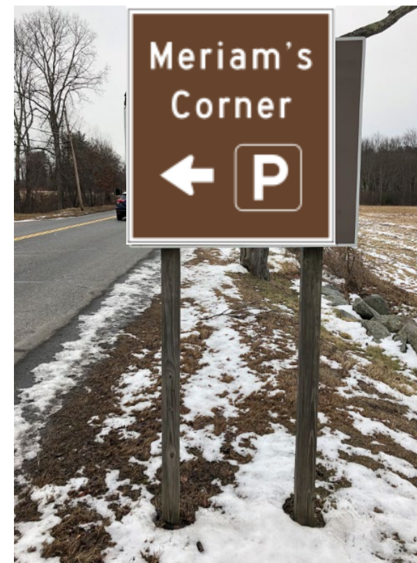
Proposed Sign 23" w x 26" ht, 3" cap or 32 x 44" 4" cap
