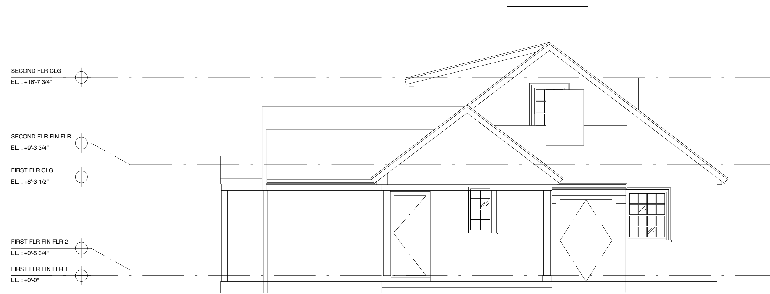
1 EXTERIOR ELEVATION: SOUTH 1/8"=1'-0"
