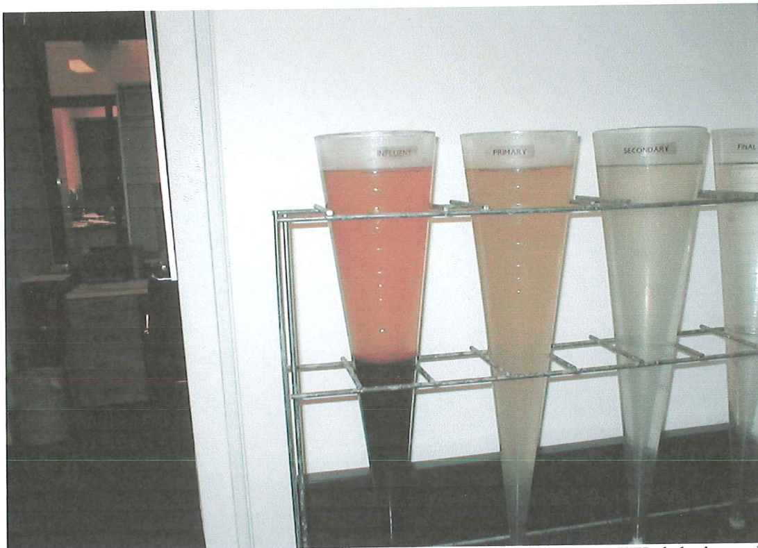
On 11/15 the settleable solids test shows the impact (high sett. solids and color) Deaconess WTP sludge has on the influent but very negligible impact on final effluent.
