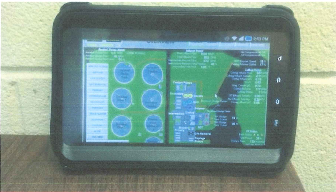
Photo: The new Samsung Tab II with VNC Viewer application viewing the Concord WWTF SCADA remotely.
